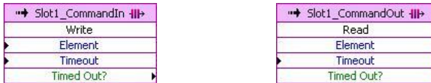
Driver internal FIFOs for data transfer between Function-VI and Driver-VI (Slot1 example)
