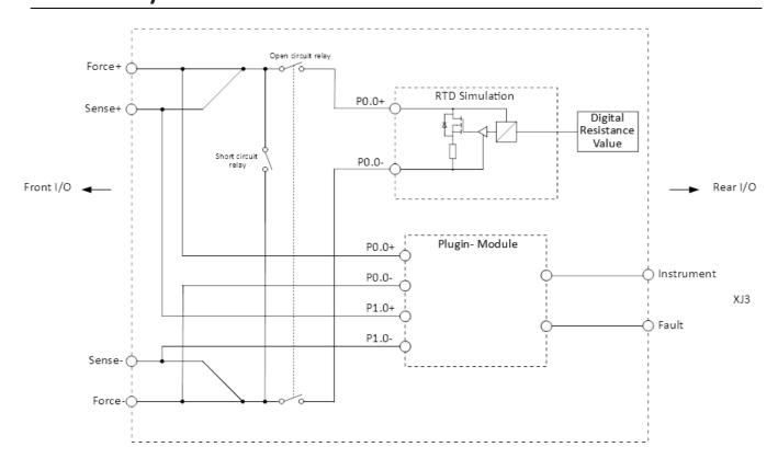
Note Diagram only shows one channel per front connector J1/J2.
